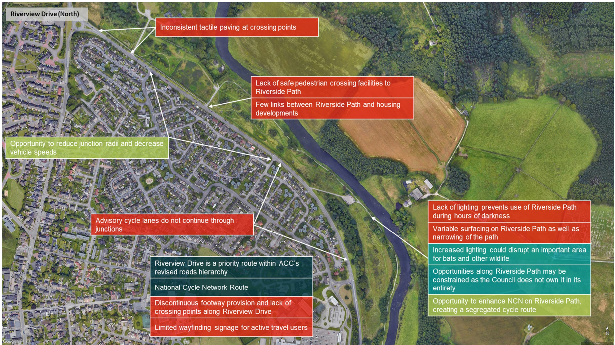
Figure 4.3: Location-Specific Issues on Riverview Drive (North) (Image Source: Google Earth)
