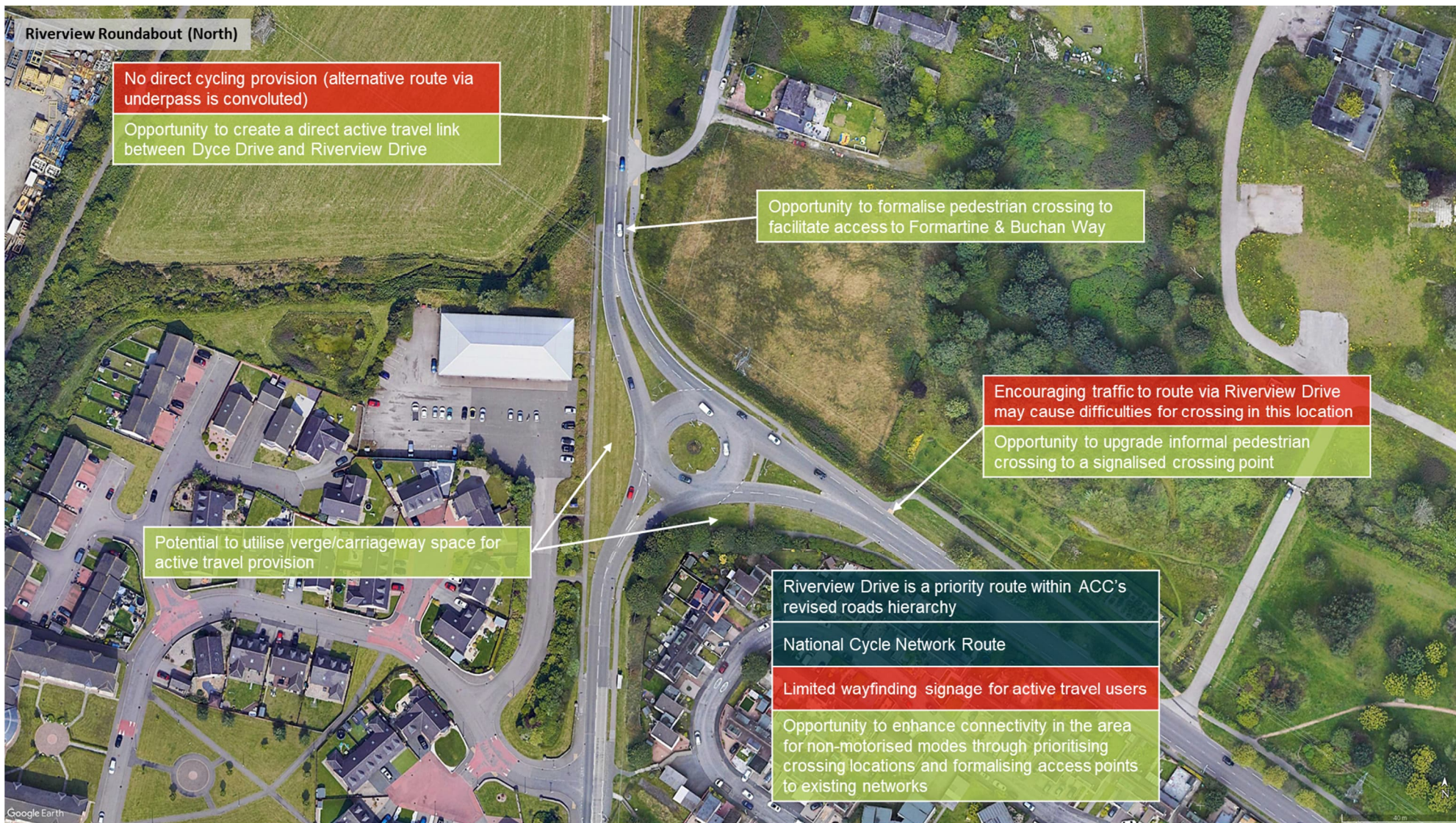
Figure 4.2: Location-Specific Issues at Riverview Roundabout (North) (Image Source: Google Earth)
